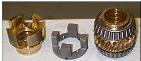
Figure 3. Follower Nut, Rotator, and Primary Nut (from left to right)
