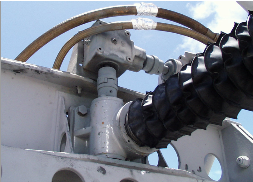
Figure 1. Current Jackscrew Used on the GOX Vent Hood
